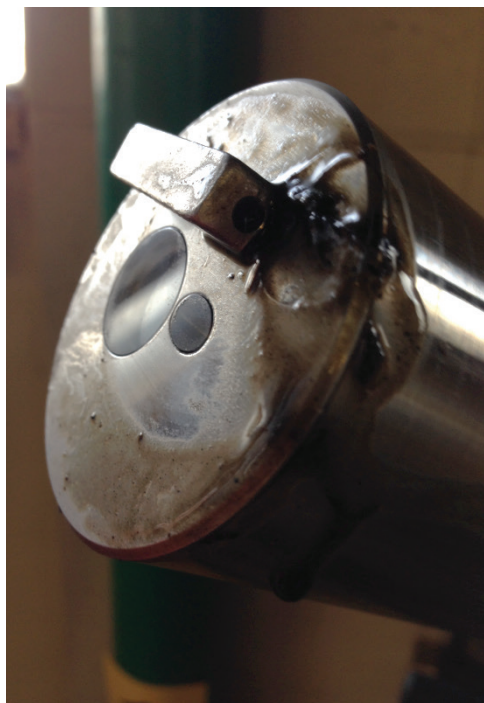
Solitax suspended solids sensor used to measure feed sludge to a centrifuge
