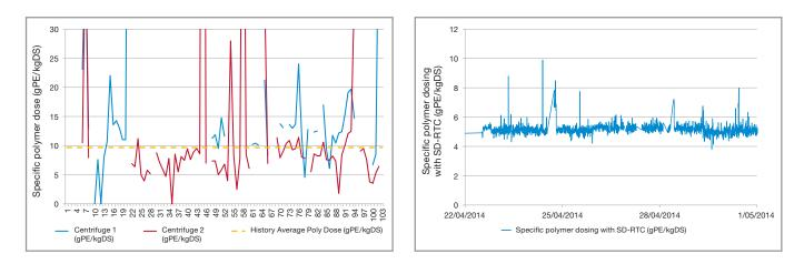
Fig. 2: Left diagram, before optimization: Very large variations in polymer dose rates leading to unsatisfactory cake quality (under dosing) and antifoam requirement due to overdosing. Right diagram, after optimization: Very stable polymer dose rates – Average 5.2 g polymer / kg DS.
